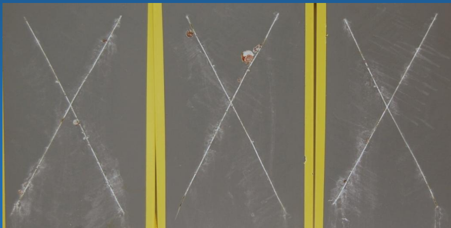
System 7: LCC2 (50ppm Cr+6)-Deft 44GN098-APC (low-chrome)
