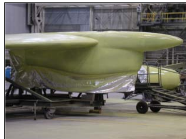
C-5 Horizontal Stabilizer Primer Application
