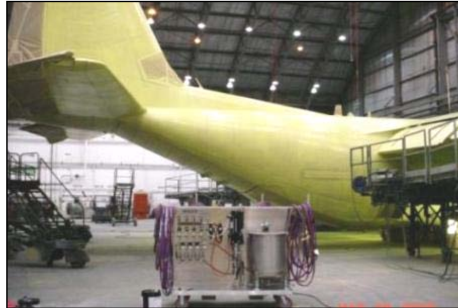
C-130 Primer Application Utilizing AAA Paint Delivery System
