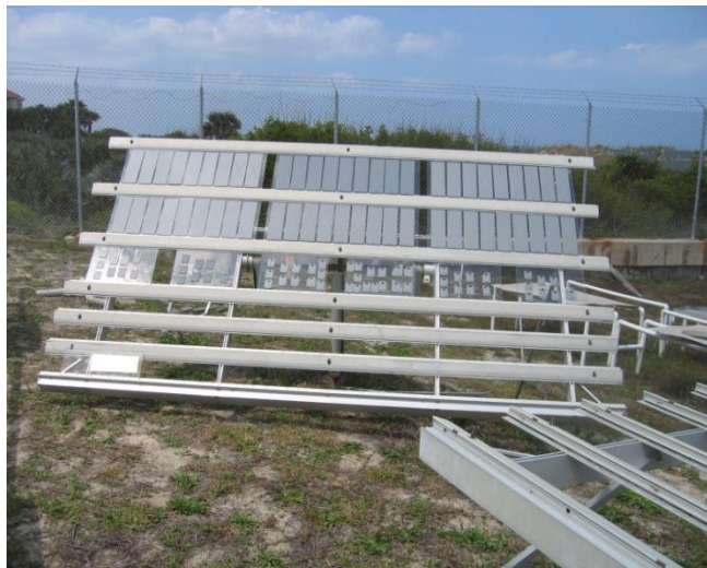
Daytona Test Rack @ 50 Meters (1 of 3 in use; ESI Steel = 165,000 microgm/cm2/yr.
