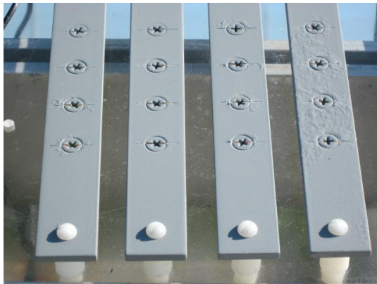
Galvanic Test Samples < 1 Year; 2024 Al/Steel
