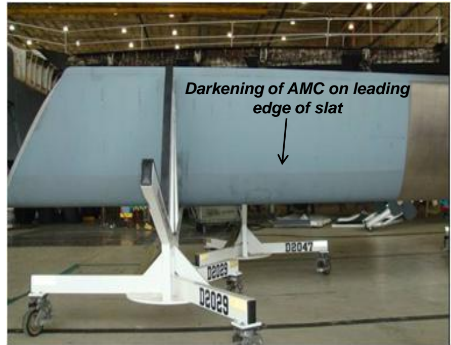
P17 slat after 956 flight hours after leading edge touch-up with AMC.
