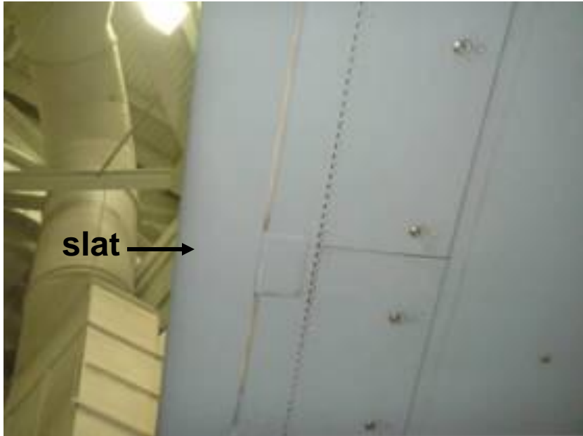
Good color match of AMC with wing
