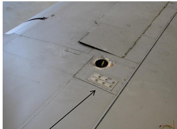
Panel with 6 sensors on C130; Upper Fuselage
